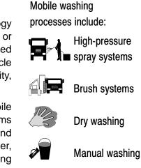
Mobile washing equipment is brought to the facility by an independent vehicle washing contractor; thus no construction is required. Typical wash water containment systems include storm drain covers, berms, or inflatable mats.
