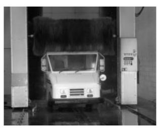
to hold detergent, surge water, and rinse water. A control system is necessary to activate the wash, control the detergent level, and time the various stages of the washing cycle. When water is reclaimed, a system to prevent algal and bacterial growth and odors in holding tanks may be required.
