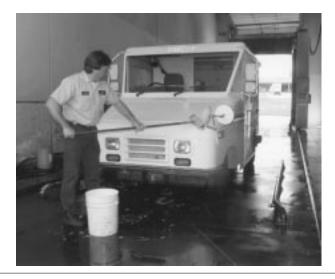
removed, these systems use any combination of cold water, hot water, or steam, with no detergent, heavy duty detergent, or acid-detergent washes. When necessary, vehicles are brushed to remove mud and dirt before the high-pressure water system is utilized. Washing times vary depending on the equipment used, how dirty the vehicle is, and how clean the vehicle needs to be. Typical washing times are approximately 10 minutes to wash an LLV and up to 30 minutes to wash a tractor-trailer.
