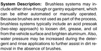
Similar to the mechanical brush systems, brushless drive-through systems require a framework consisting of free-standing arches: an acid presoak applicator arch, a detergent arch, and a high-pressure rinse arch. Brushless gantry systems have a single rolling arch.
