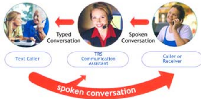
Figure A. VCO allows a caller to speak and receive typed responses from the other party (via a Telecommunications Relay Service communication assistant or relay officer).
