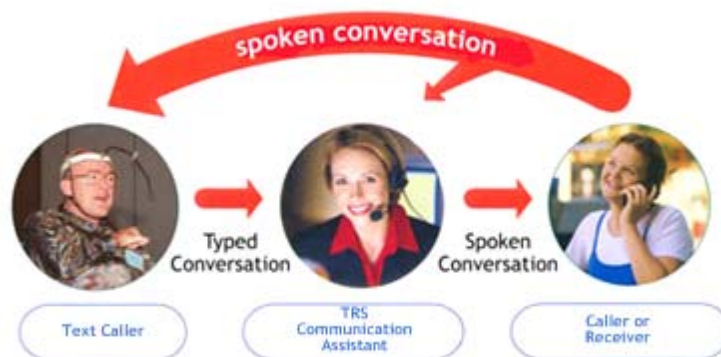
Figure B. HCO allows a caller to type conversation (relayed through a Telecommunications Relay Service communication assistant or relay officer), then hear spoken responses from the person they are calling.
