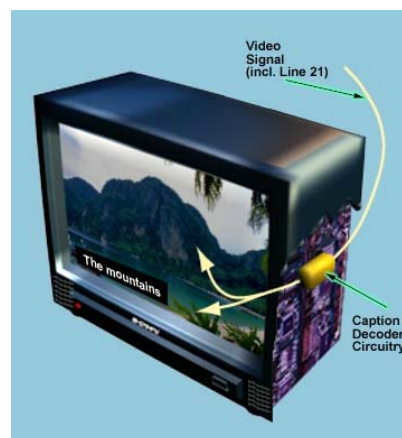
Exhibit 8-2.1: A diagram showing a video signal (including Line 21) being received and interpreted and played back by Caption Decoder Circuitry in a television display or computer monitor.
